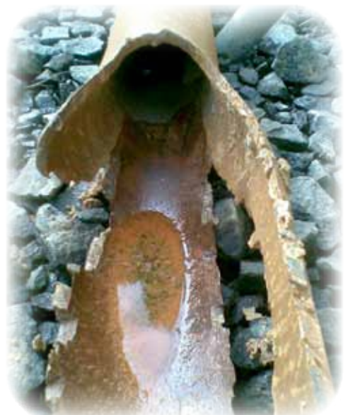
▲ Exploded drill rod to recover drill string
