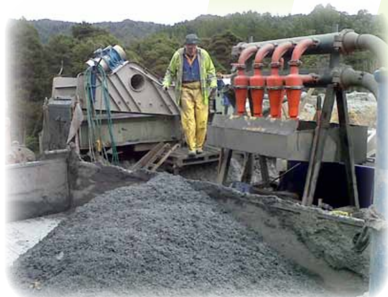
▲ Tunnel cuttings removed from the fluid with 3 shaker screens and 16 hydro cyclones
