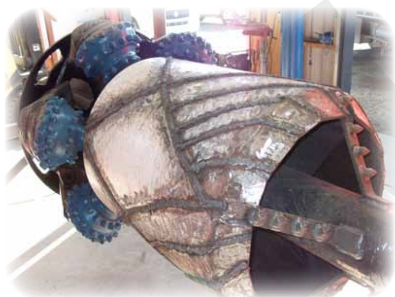
▲ 1050mm diameter tunnel requiring three reamer passes
