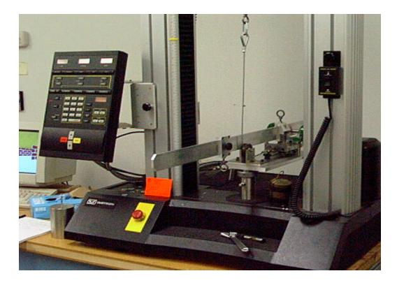
FIGURE 2- Shear scratch resistance test apparatus
