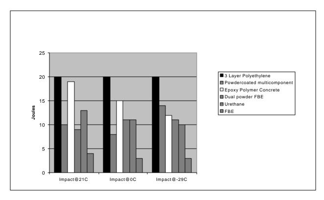
FIGURE 7- Impact Resistance results for anti-abrasion coatings
