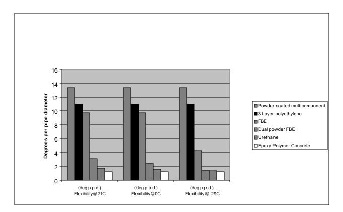
FIGURE 6- Flexibility results for anti-abrasion coatings
