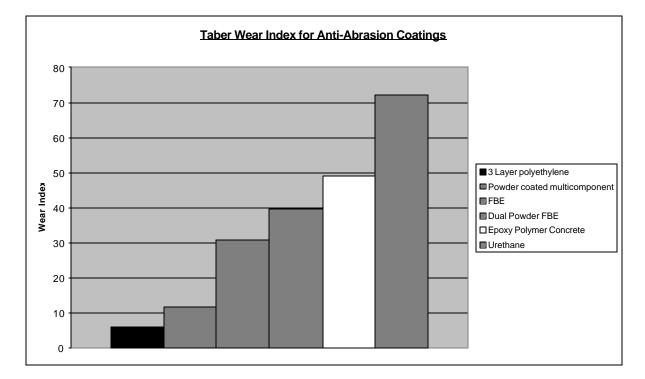
FIGURE 5- Taber Wear results for anti-abrasion coatings
