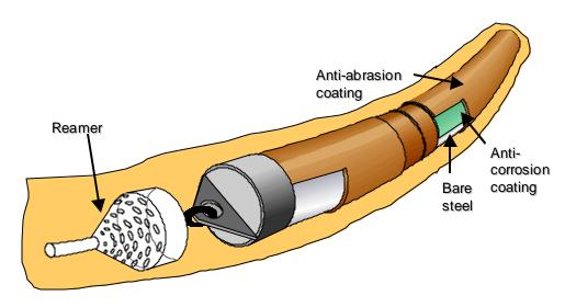
FIGURE 1- Schematic of pullback of pipeline in a HDD crossing
