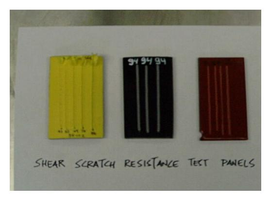
FIGURE 3- Shear scratch resistance test panels
