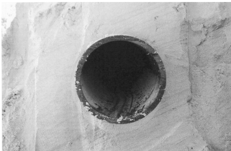
Fig. 13. 200 mm (8 in.) sand excavation at 1 year
