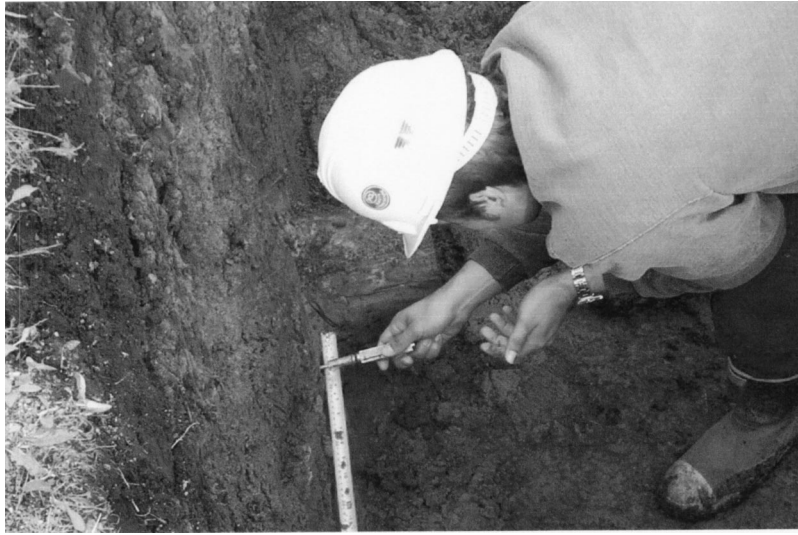
Fig. 14. Field measurement of unconfined shear strength of annular space
